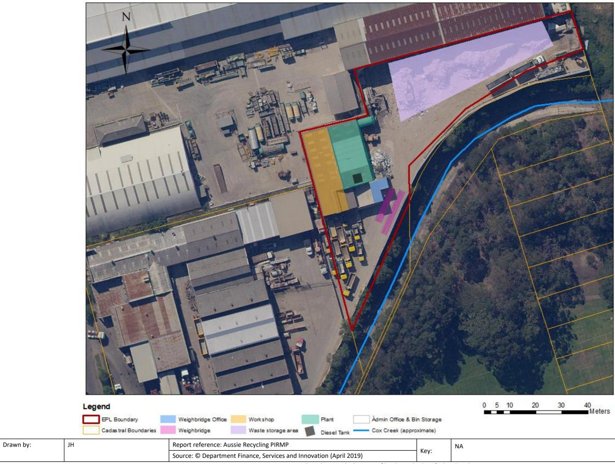
Figure 2: Site plan, showing the location of key hazards identified in this Plan.
